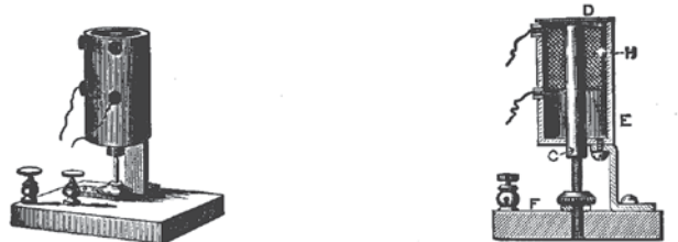
Figure 5: Bell's "iron box" receiver, as taken from Bell's Deposition in the Suit to annul the Bell patents, titled The Bell Telephone , Boston: American Bell Telephone Co., 1908, at page 100.
